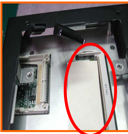
Single-sided IC used the 2.0mm thickness thermal pad.
