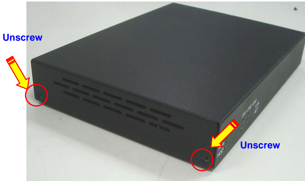
(a) Unscrew left side screws of chassis top cover
