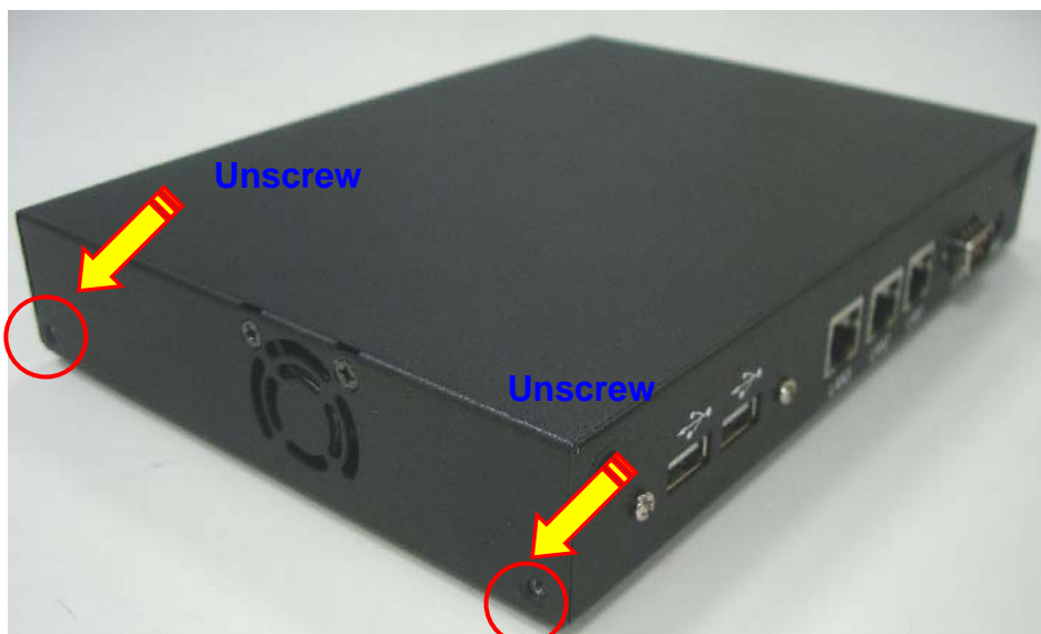
(b) Unscrew right side screws of chassis top cover
