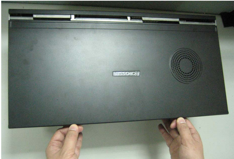
Fig-04 Lock the top cover
