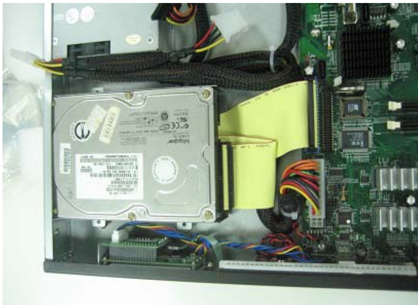
Fig-03. Lock HDD bracket with IDE cable
