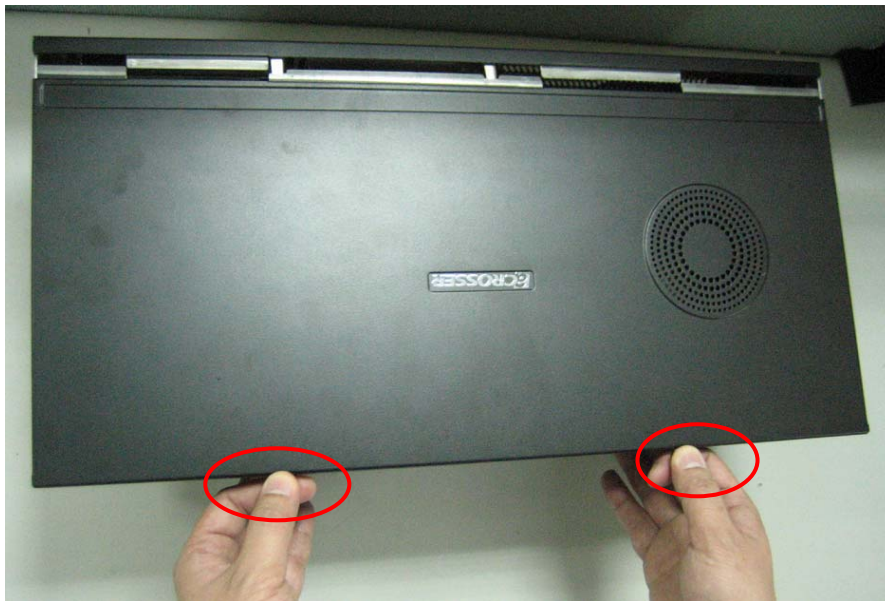
Fig. 01 Remove the top cover
