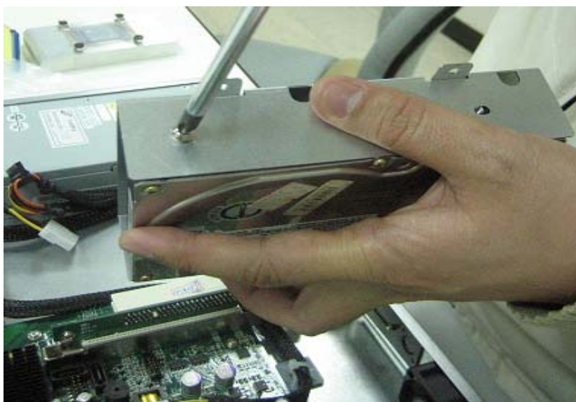
Fig-02 HDD bracket with HDD body
