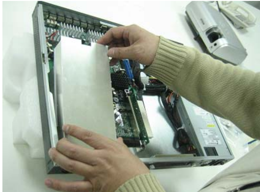
Fig-11 Take off the air flow cover
