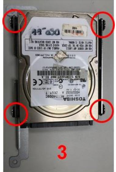
Step 3: Install the HDD Bracket & Cable and fix the screws.
