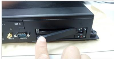
Step 4: Push the latch left, a red circle appears. The door is locked.
