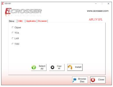
Step 2: Click the "**Select All**" button to select all the driver checkboxes, and then click "**Install**" button to start installing all the selected drivers.
