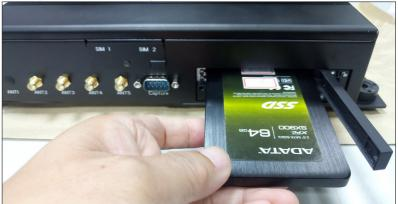
Step 3: Firmly close the door so that the SSD will be slided into its contact position. (Failing to do so could cause a loose contact with the SSD.)
