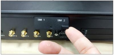
Step 3: Insert your SIM card. Secure the cover plate.
