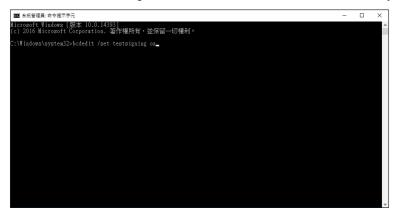
To shutdown the Windows test mode, run the command "BCDEdit /set testsigning off", and restart the system.
