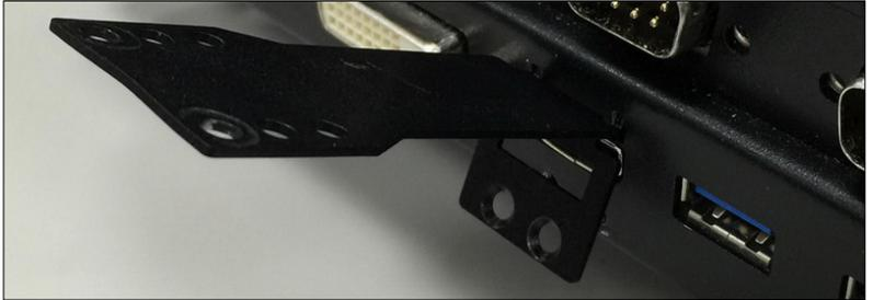
Step 2: Lock the HDMI locking-bracket with the two black screws that came with the package.
