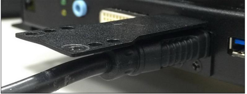
Step 5: Fasten the HDMI cable-end with a cable-holder. Lock the cable-end to the bracket with this cable-holder by two white screws that came with the package. (There are two types of cable-holder provided: 4mm and 7mm. Use the type 4mm for HDMI cable of thinner than 6mm in diameter. Use the type 7mm for HDMI cable of thicker than 6mm in diameter.)
