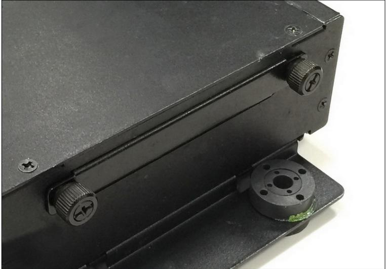
Step 2: Lock the disk with 4 screws provided in the package.
