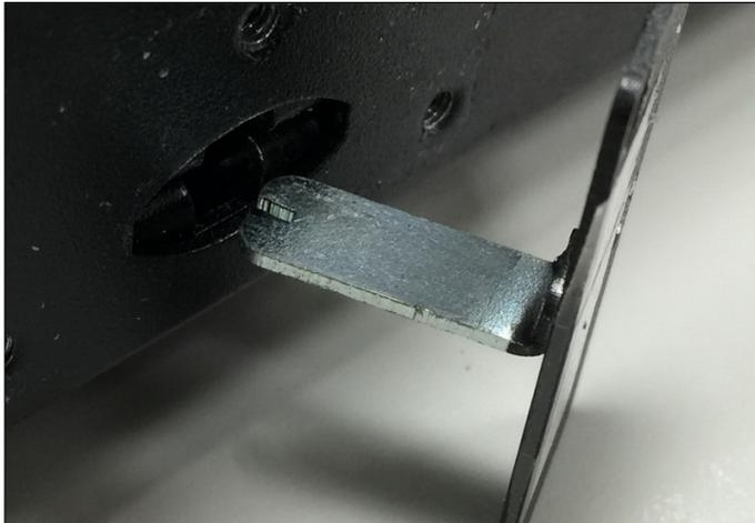
**Note:** To remove the SIM card, turn the cover-plate 90 degrees and stick it into the slot. Push the SIM card inward and then release. The card bounce outward a little bit. Use a tweezers to pinch the card out.
