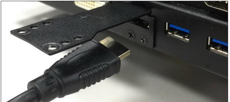
Step 4: Firmly push the HDMI cable all the way into the socket.
