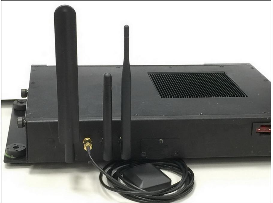
The antennas shown for installation demonstration in this photo from left to right are: AUX (Reserved with a cap covered), 4G LTE, GPS, Bluetooth, WiFi.
