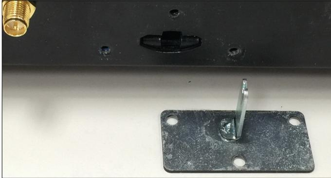
Step 3: The SIM card cover-plate is mechanically designed to fit for pushing in the SIM card into its position. Turn the cover-plate 90 degrees to push the SIM card into its position.
