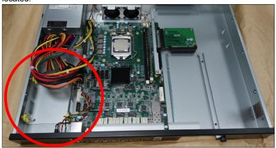
Step 2: Remove the four screws that fasten the HDD bracket from the chassis bottom cover.
