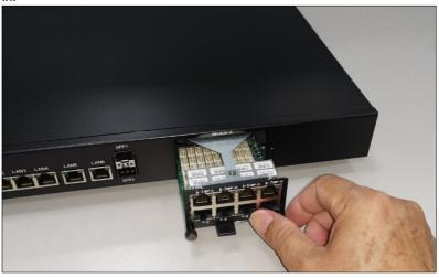
Step 4: Push the latch left. This will lock the module.
